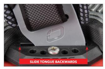
SLOWLY UNDO THE BASEPLATE SCREWS (DON'T UNSCREW ALL THE WAY) TO ALLOW CLEARANCE FOR THE STRAP TONGUE TO BE PUSHED DOWN, THEN MOVE THE TONGUE FORWARD OR BACKWARD IN THE BASEPLATE SLOT, THEN PULL IT BACK UP INTO PLACE.
